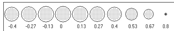
Figure 2: Solution space consisting of 818 voxels (shown as dots) corresponding to a 3D regular cubic grid with minimum inter-voxel distance d=0.133 , confined to a maximum radius of 0.8, with vertical coordinate values z \geq -0.4 . Numbers below each horizontal "brain" slice indicate the Cartesian "z" coordinate. Coordinate origin is at sphere center.
